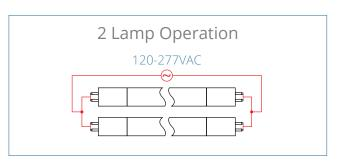
**NOTE**: both pins on each end of lamp must be connected to line voltage as shown above. If lamp holder is a "non-shunted" (T12) type, it must be shunted (shorted) by external jumper. Most T8 lamp holders are internally shunted and will not require an external jumper.
